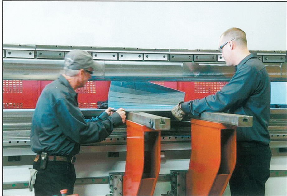
BMC Fabrication Services employees Perry Farris, left, and Kyle Carrier form a reducer cone on a new press brake for a material handling and ductwork customer at the Columbia business. (Courtesy photo)
